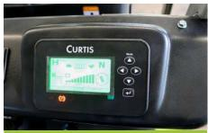
With multi-function LCD display users can easily monitor the performance and working status of the vehicle through the information displayed on the display.
