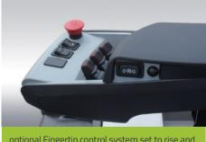
optional Fingertip control system set to rise and fall, forward, backward, lateral and emergency stop switch, a horn, lighting control and other control buttons in one.
