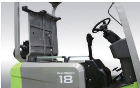
Advanced suspension seat with suspension damping function, which can ease the driver fatigue, and improve work efficiency.
