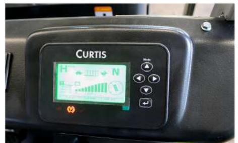
With multi-function LCD display users can easily monitor the performance and working status of the vehicle through the information displayed on the display.
