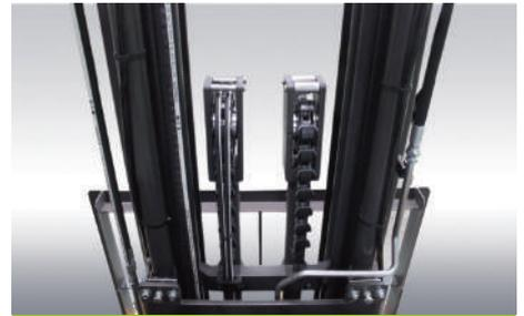
Mast triple full free equipped with double front cylinder, increasing greatly the driver operating field of vision.
